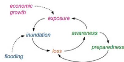
Figure 1: Representation of the coupled human-flood system as encoded in the socio-hydrological flood risk model. The model accounts for dynamics in hazard (blue), exposure (pink), and vulnerability variables (green) to continuously assess flood loss (orange)
